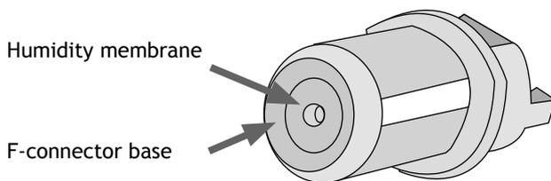
The Signia housing has been tested under 1 meter of water for 30 minutes, corresponding to the IPx7 requirements. No water penetrated into the housing with the glue sealing, so the sealing between the backplate and the housing, and the sealing between the F-connector and the housing are both water tight to at least 1 meter.
