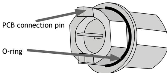
To ensure that potential corrosion over a long period of time does not affect the the electrical performance, the outer shield of the F-connector is soldered directly onto the printed circuit board (PCB). This is an improvement to the norm where the outer shield of the F-connector is part of the housing and through soldering pins connected to the PCB. But the housing can be vulnerable to electrolytic corrosion as
