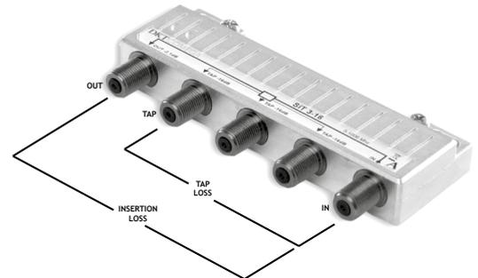
A signal is applied to the IN connector. For Tap Loss the output is measured on the other TAP connectors. For Insertion Loss the output is measured on the OUT connector.
