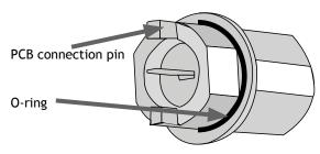
To ensure that potential corrosion over a long period of time does not affect the the electrical performance, the outer shield of the F-connector is soldered directly onto the printed circuit board (PCB). This is an improvement to the norm where the outer shield of the F-connector is part of the housing and through soldering pins connected to the PCB. But the housing can be vulnerable to electrolytic corrosion as
