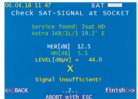
One of the wizards: simple and guided check of the signal quality at the antenna socket.
