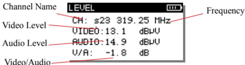
Figure 4-1-1 Analog Signal Measurement
