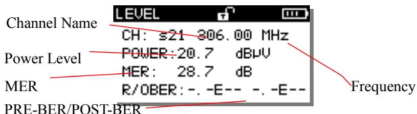
Figure 4-1-2 Digital Signal Measurement Interface
